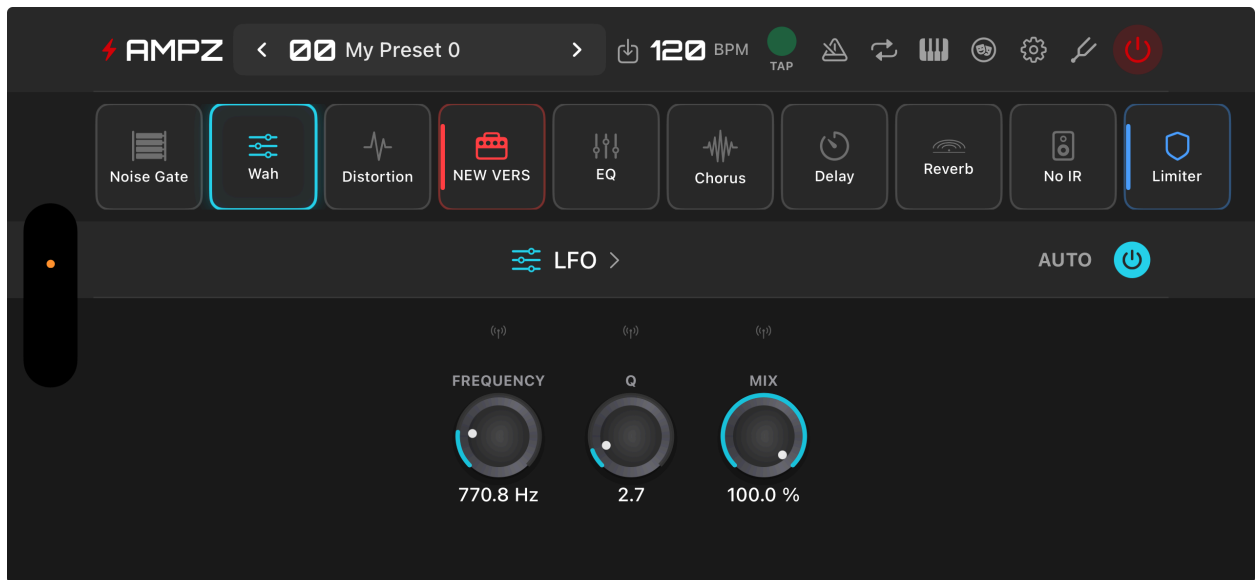
Figure 30: Wah with Auto OFF — manual frequency control
