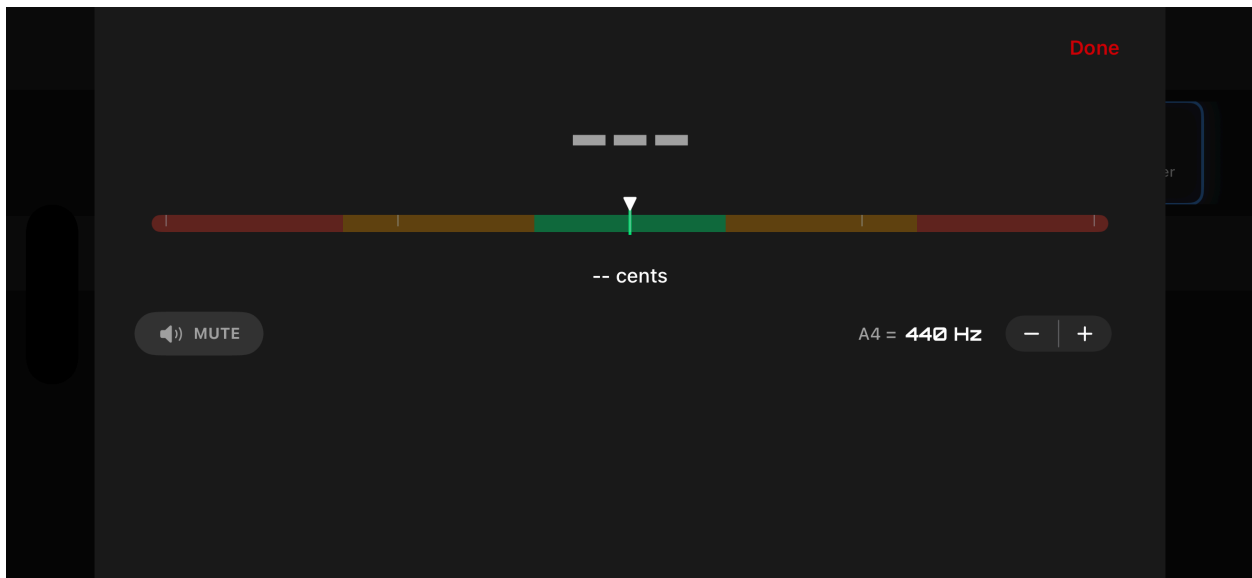
Figure 47: Tuner — note display, cents gauge, and mute control
